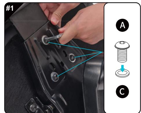
Install the backrest to the tilt mechanism. Be aware that the placement should be correctly aligned. Use the screws and iron washers to make sure the backrest is securely fastened.
