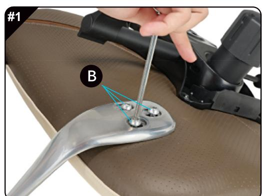
Install the armrests onto the bottom of the cushion. Use the screws to make sure they are securely fastened.
