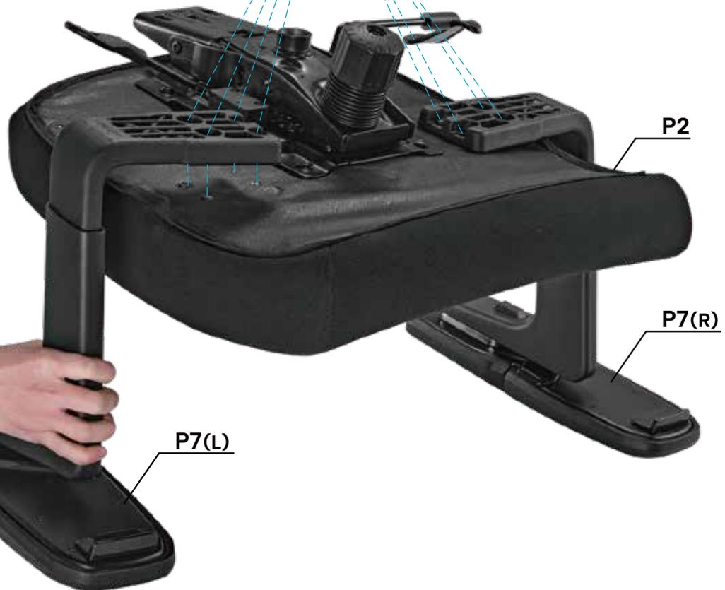
Install the armrests (P7) onto the bottom of the cushion (P2). Use the screws (C) and gaskets (E) to make sure they are securely fastened. Note: distinguish between the left and right installation positions of the armrests.
