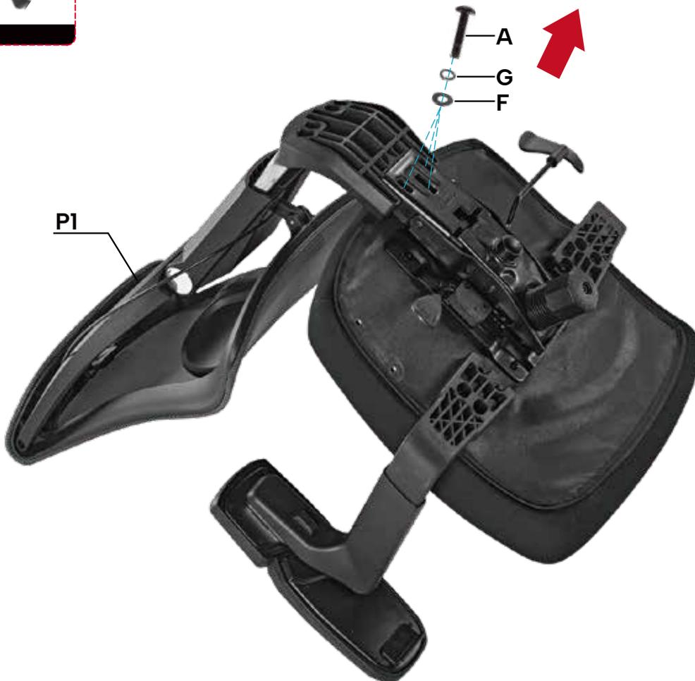
Install the backrest (P1) to the tilt mechanism (P8). Be aware that the placement should be correctly aligned. Use the screws (A), gaskets (F) and iron washers (G) to make sure the backrest is securely fastened.
