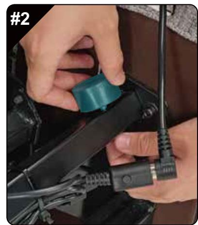
First, screw out the nut, and then insert the anti-collision cushion into the metal frame, finally fasten it with the nut.
