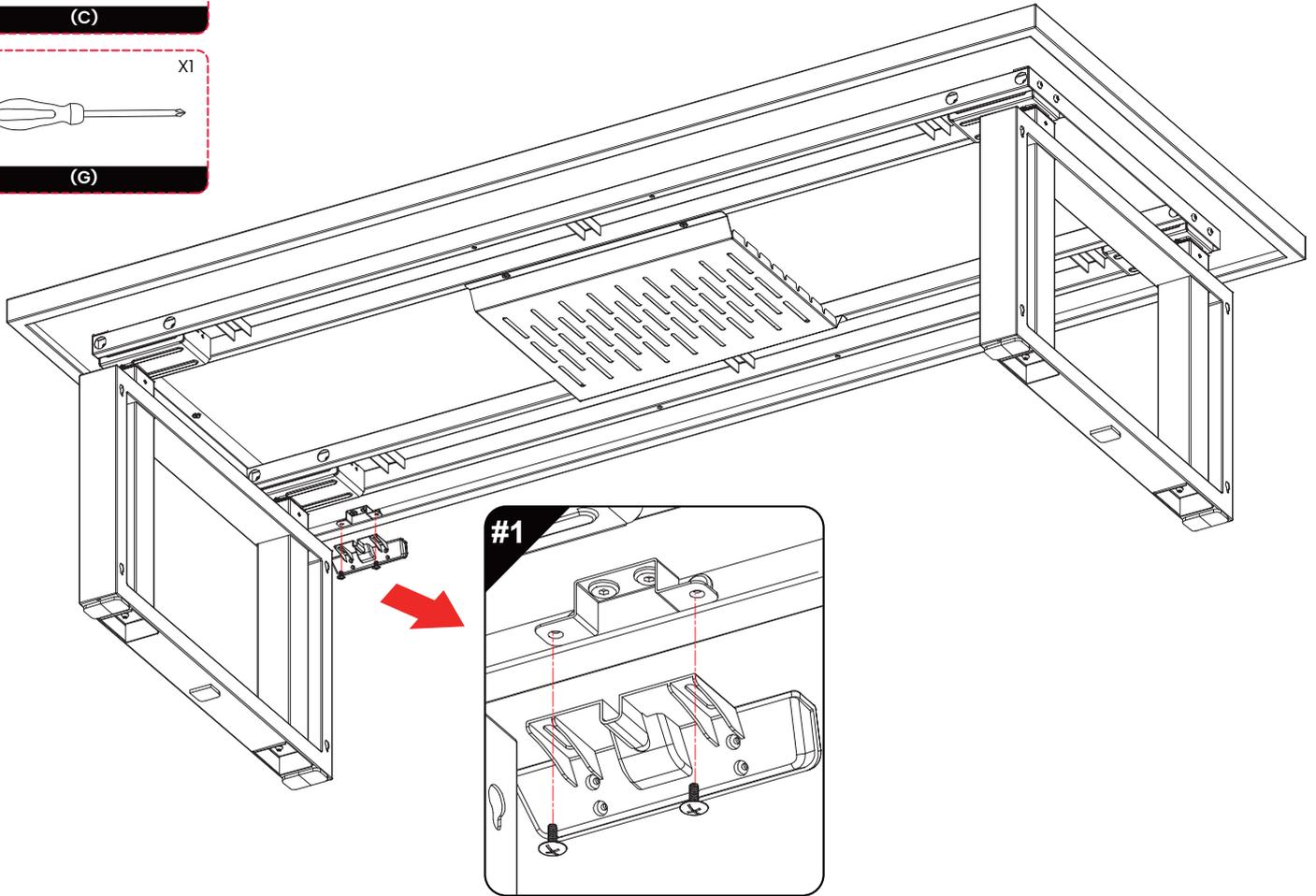
Tie the cable with the cable management buckle.
