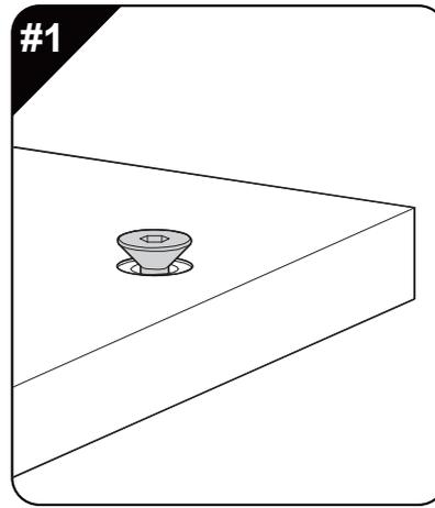
Don't screw in, leave the rod length of about 1mm.
