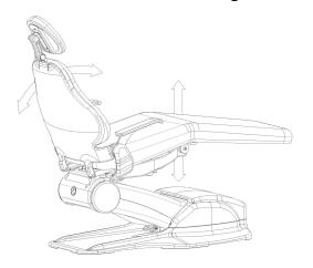
Manual positioning of the chair can be done by operating the footswitch or by the touchpad control located at the delivery system tray.
