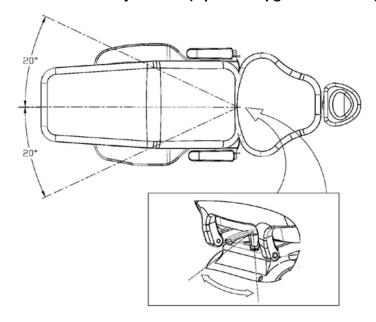
Release the chair rotation lock by turning the hand lock to the right. The chair could manually rotate approximately 20° to either side of its center position. To secure the final position, simply turn the hand lock to the left.
