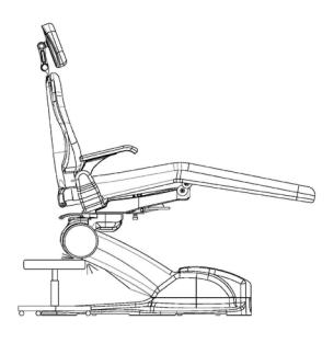
To prevent damage to the chair or other equipment, all FDC dental chairs are equipped with a Collision Protection System.
