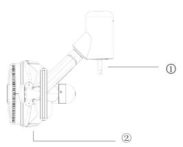
There are two joint connections to allow better angle/location adjustments of the dental light. The dental light can be adjusted to the ideal location during operation. The dental light is equipped with a proximity switch for ON/OFF control and brightness level adjustment.
