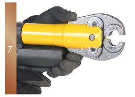
Insert the correct size press jaw for the size of fitting being pressed. Ensure jaw is clean and moves freely.
