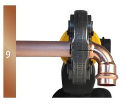
Press the trigger on the tool, hold down until jaws fully close and an audible click is heard. This completes the pressing process.
