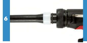
Repeat 6 rotations for 16mm and 8 rotations for 20mm until snug against the expander head. Remove tool from pipe end.
