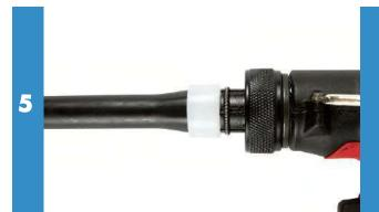
Press and hold the trigger on the expander tool, the expander head will begin to splay and expand the end of the pipe. The expansion tool comes with built-in auto rotation. Ensure you hold the pipe whilst expanding. Let the tool complete its cycle, do not stop and start.
