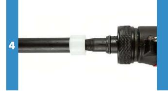
Choose the correct size expander head for the pipe being expanded. Pictured is the 20mm head suitable for 20mm pipe. Gently, insert the expander head into the end of the pipe.
