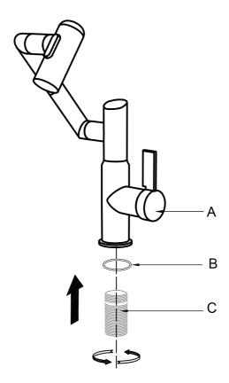
Install the waterproof rubber ring (B) and the threaded metal pipe (C) on the faucet body (A) in sequence.
