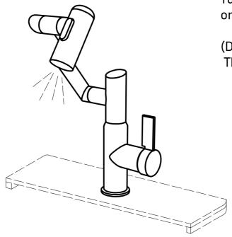
Turn on angle stops, turn the faucet on and check for leaks.
