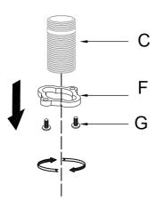
Shut off the water supply. Remove the old faucet. Clean the mounting surface. Remove mounting hardware (F & G) from threaded metal pipe(C).
