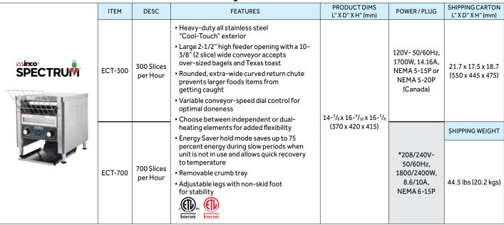
Easy-load rack with large & high feeder opening accepts over-sized bagels and Texas toast
