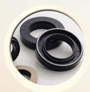
NAK AP Seal is created for heavy-duty applications especially where seal (such as TC) that consists of a spring loaded radial sealing lip and a static dust lip often falls short in heavy duty and at the same time heavy contaminated applications. In many cases the failure is caused by the penetration of mud and water at the radial lip. NAK AP Seal resolves this problem by providing the optimal protection against mud, water and other contaminants through a variety of design features.
