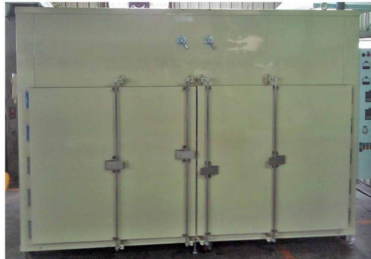
Precision hot-air oven is specially made for sulfurization and formation of large-sized rubber products.
