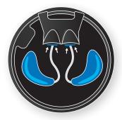
**CAUTION:** Ensure there is nothing in or on the chamber seal that will prevent the lid from closing. Do not put anything in the chamber that will hit the inside of the lid, as this will prevent a seal on the chamber and reduce effectiveness of the drying process.
