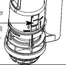
To adjust the part flush volume, move slide up for less and down for more.
