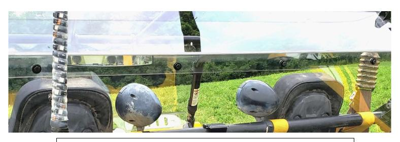
USE BOLT WITH SMALL WASHER ON THE OUTSIDE, SECURE WITH SMALL WASHER AND LOCK NUT ON THE INSIDE.
