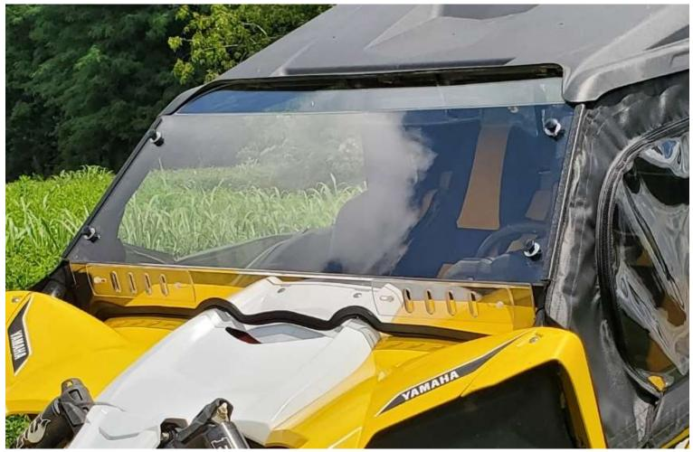
**Step 9:** Tighten the knob bolts holding the windshield in place. **DO NOT OVER TIGHTEN THE KNOB BOLTS. NEVER USE THE KNOB BOLTS TO PULL THE CLAMPS TO THE WINDSHIELD.** If the clamps need to be re-positioned, loosen the clamp nuts to do so.
