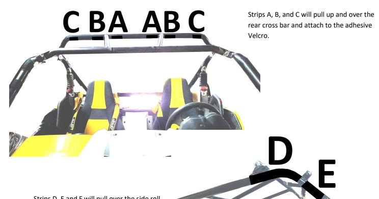
Strips D, E and F will pull over the side roll bar and attach to the adhesive strips.
