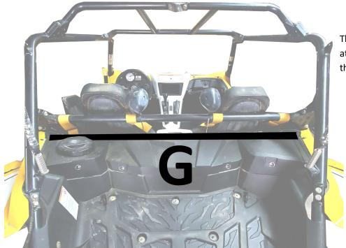
The bottom of your back panel will attach to strips G all the way across the front of the bed.
