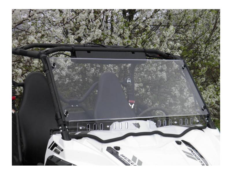
**Step 7:** When satisfied that the windshield is positioned properly, tighten the two nuts on the back side of each clamp.
