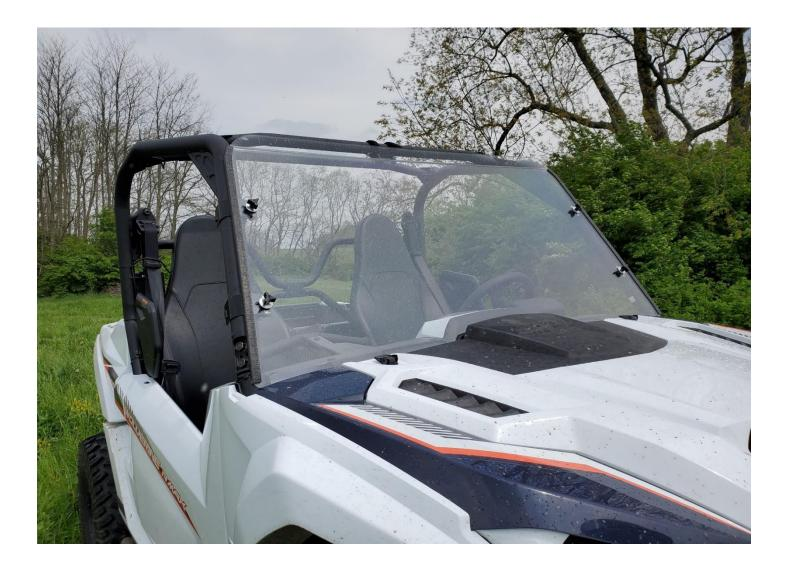
**Step 7:** When satisfied that the windshield is positioned properly, tighten the two nuts on the back side of each clamp.
