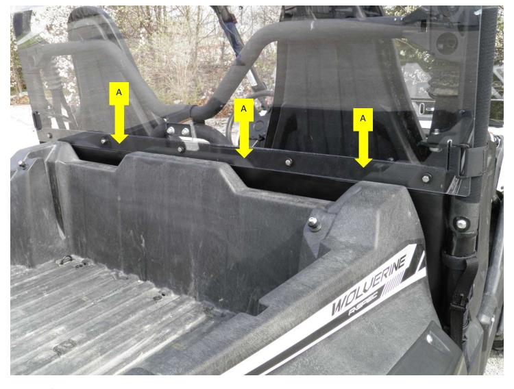
**Step 3:** After the velcro is attached to the polycarbonate anchor strip, holes will need to be cut to match the holes in the anchor strip. The canvas lower back panel will then velcro to the anchor strip so that the holes line up. The polycarbonate anchor strip is then attached to the inside of the polycarbonate back panel and secured with the included bolts and hardware.
