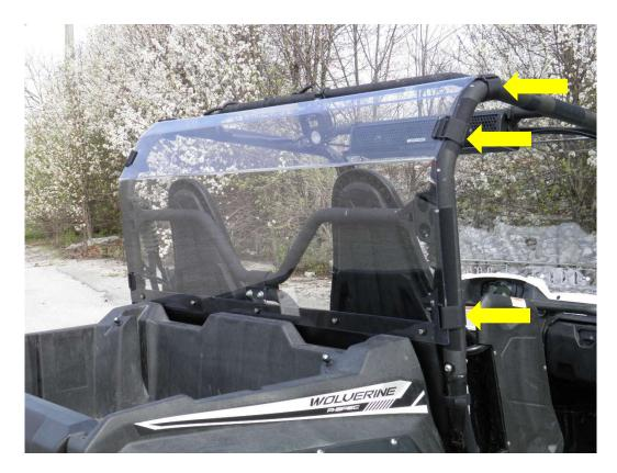
**Step 5:** On each side of the back panel, feed a Quick Attach Strap into the slot in the windshield from the outside. Please note, the "Velcro" side of the strap should face inward. Wrap the strap around the roll bar and feed it through the buckle. Pull the strap tight and adhere the hook end of the strap to the loop strap.
