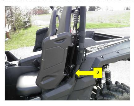
**Step 8:** Wrap the sewn-in velcro in the middle of the canvas lower back panel around the bar between the seats.
