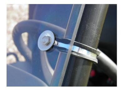
**Step 4:** When satisfied that the windshield is positioned properly, tighten the nuts on each clamp.
