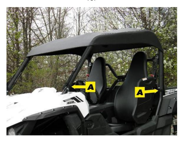
**Step 5:** After all adhesive hook strips are attached, begin attaching the enclosure to the cab frame. As you attach the hook and loop, square each panel to the frame. **PLEASE NOTE, FOR MAXIMUM ADHESION, ALLOW THE ADHESIVE HOOK TO ADHERE TO THE FRAME FOR 24 HOURS BEFORE PULLING AGAINST THE HOOK WITH THE LOOP STRIPS.**
