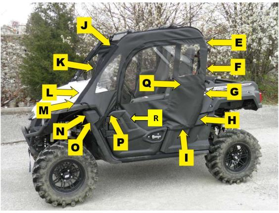
**Step 4:** After all adhesive hook strips are attached, begin attaching the enclosure to the cab frame. As you attach the hook and loop, square each panel to the frame. **PLEASE NOTE, FOR MAXIMUM ADHESION, ALLOW THE ADHESIVE HOOK TO ADHERE TO THE FRAME FOR 24 HOURS BEFORE PULLING AGAINST THE HOOK WITH THE LOOP STRIPS.**
