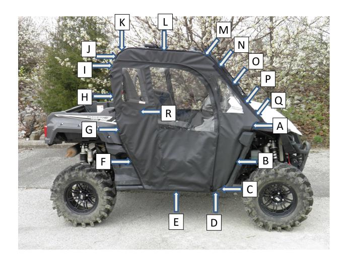
**Step 4:** After all adhesive hook strips are attached, begin attaching the enclosure to the cab frame. As you attach the hook and loop, square each panel to the frame. **PLEASE NOTE, FOR MAXIMUM ADHESION, ALLOW THE ADHESIVE HOOK TO ADHERE TO THE FRAME FOR 24 HOURS BEFORE PULLING AGAINST THE HOOK WITH THE LOOP STRIPS.**
