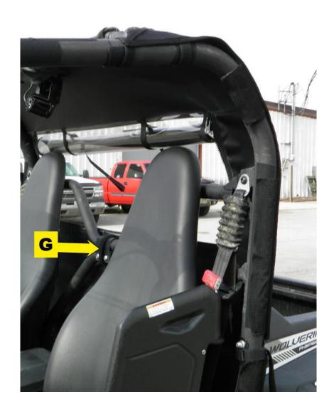
**Step 3:** After all adhesive hook strips are attached, begin attaching the enclosure to the cab frame. As you attach the hook and loop, square each panel to the frame. **PLEASE NOTE, FOR MAXIMUM ADHESION, ALLOW THE ADHESIVE HOOK TO ADHERE TO THE FRAME FOR 24 HOURS BEFORE PULLING AGAINST THE HOOK WITH THE LOOP STRIPS.**
