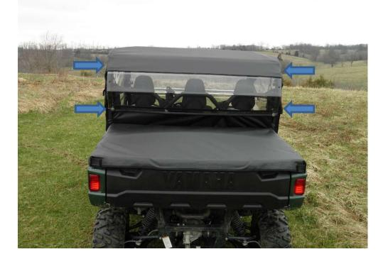
**Step 5:** When satisfied that the back panel is positioned properly, tighten the nuts on each clamp.
