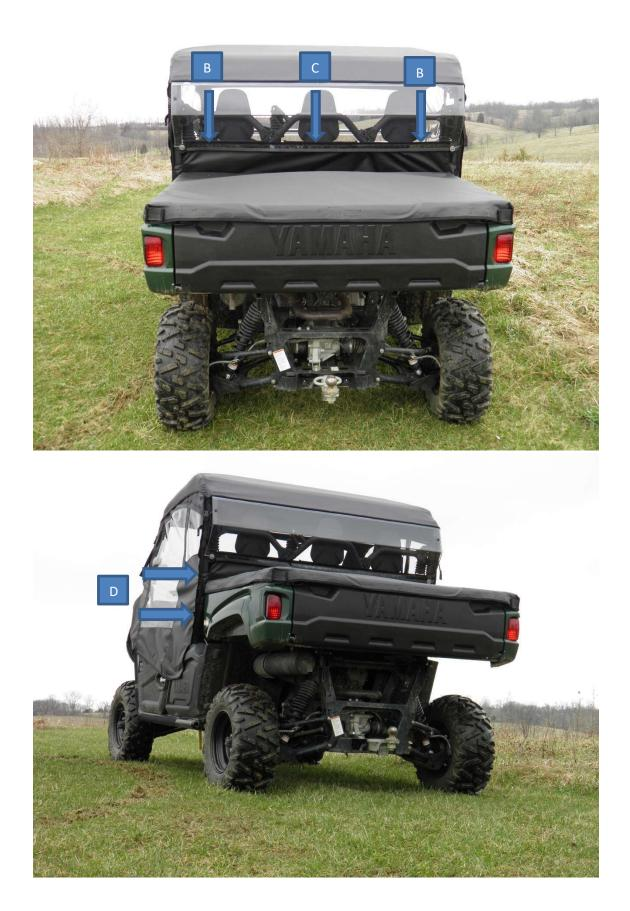
**Step 3:** One at a time, open a clamp and wrap around the rear roll bars corresponding to the picture shown below. The flat side of the loop clamps should face forward with the bolt hole openings on the inside of the roll bars.
