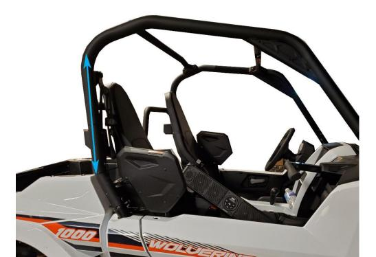
MAGNETS WILL SNAP TO ROLL BAR WHEN ZIPPING THE DOOR CLOSED
