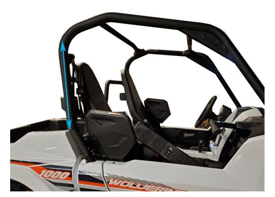
MAGNETS WILL SNAP TO ROLL BAR WHEN ZIPPING THE DOOR CLOSED
