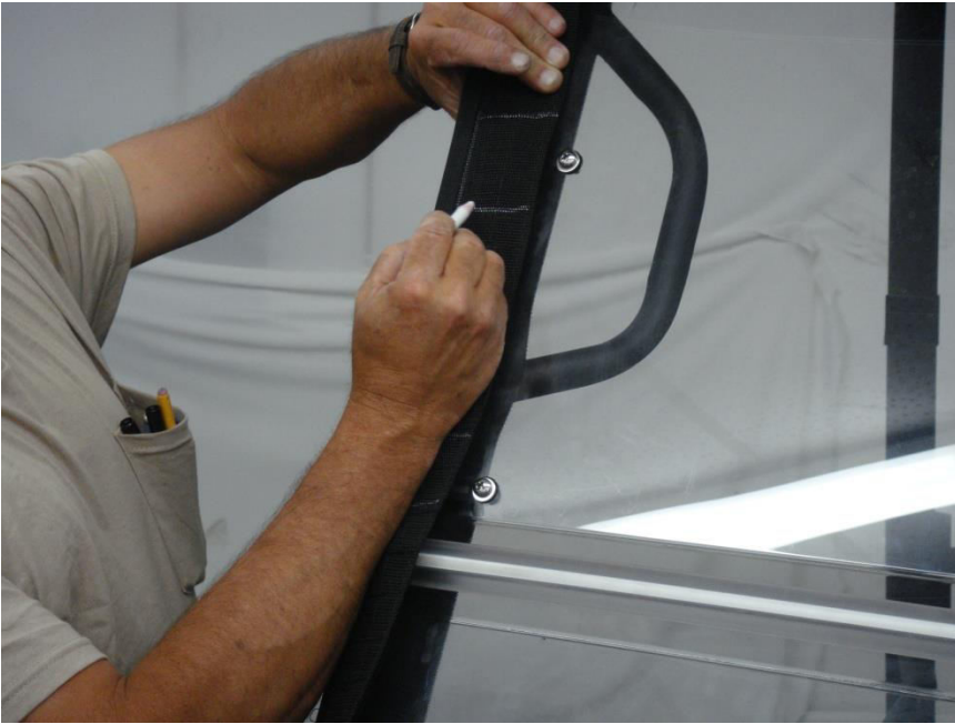
Figure 13.2 - Mark the Windshield Velcro Tabs for hard windshield Clamp locations
