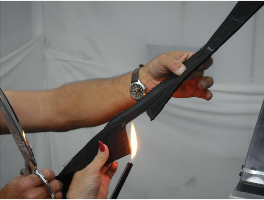
Figure 13.4 - Carefully burn the frayed thread around the cut area with a lighter.
