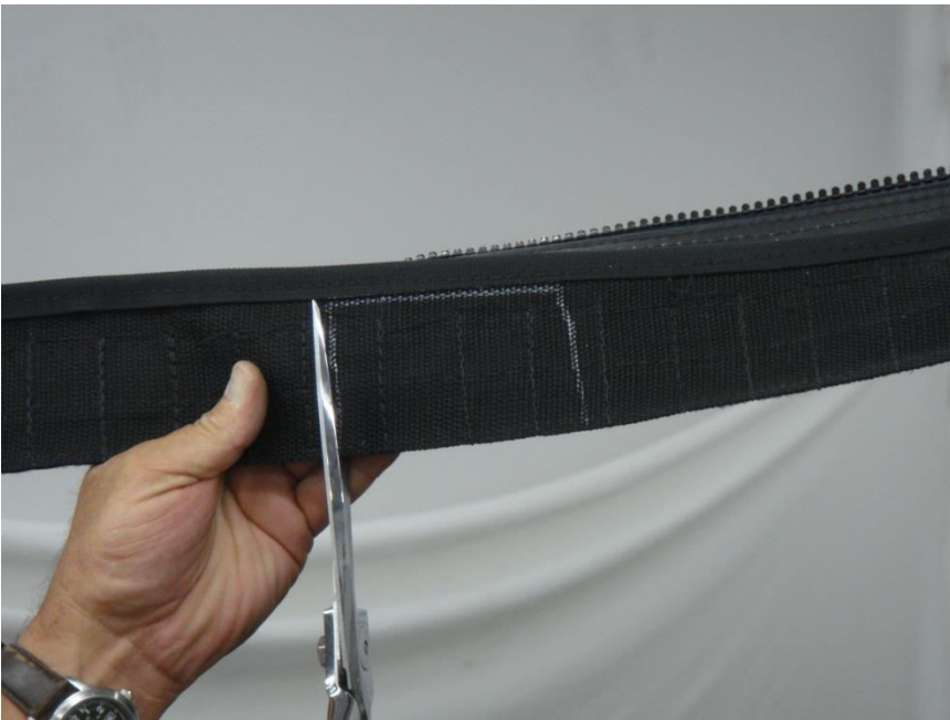
Figure 13.3 – Cut a 2” section out around where your clamps will be positioned on the Velcro Tab – be careful not to cut the binding
