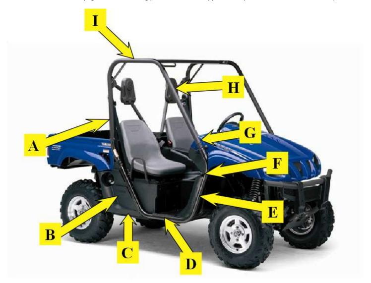
**Step 4:** After all adhesive Velcro strips are attached, begin attaching enclosure by first squaring the back of the enclosure to the rear of the cab frame and attaching the sewn-in Velcro loop to the 42" adhesive strip at the base of the back panel.
