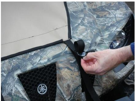
**Step 7:** Starting with the top Front Roll Bar Post Enclosure tabs pull outward and downward attaching tabs to 8" inch Velcro Strips on the Roll Bar as shown in figure 14.1. Repeat this process with the lower Front Roll Bar Enclosure Tabs making sure that the Windshield is centered between the Roll Bar posts.
