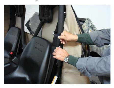
Pulling upward & outward on the 6" Rear Roll Bar Post Enclosure Velcro Tabs, attach Rear Roll Bar Post Enclosure tabs to installed 6" Velcro Strips as shown.
