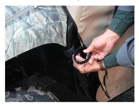
Attach front side lower Roll Bar Frame Velcro Tabs to installed 6 inch Velcro Strips by wrapping the tab around the Roll Bar Frame and Velcro Strip as shown.
