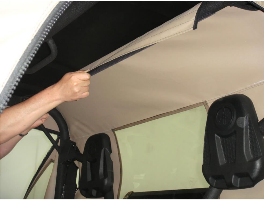
Figure 8.1 – attach 41" Rear Roll Bar Cross-member Velcro Tab
