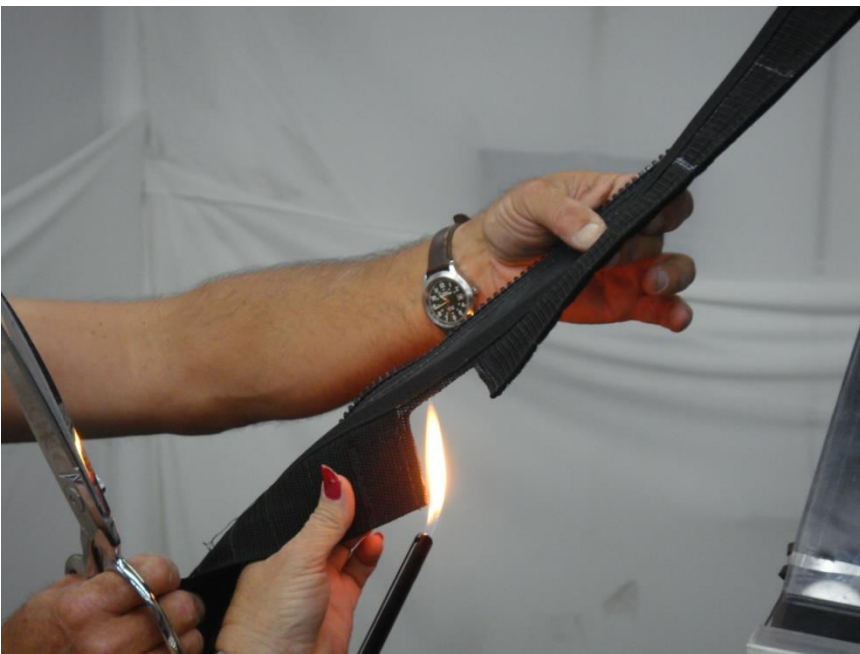
Figure 7.4 – Carefully burn the frayed thread around the cut area with a lighter.
