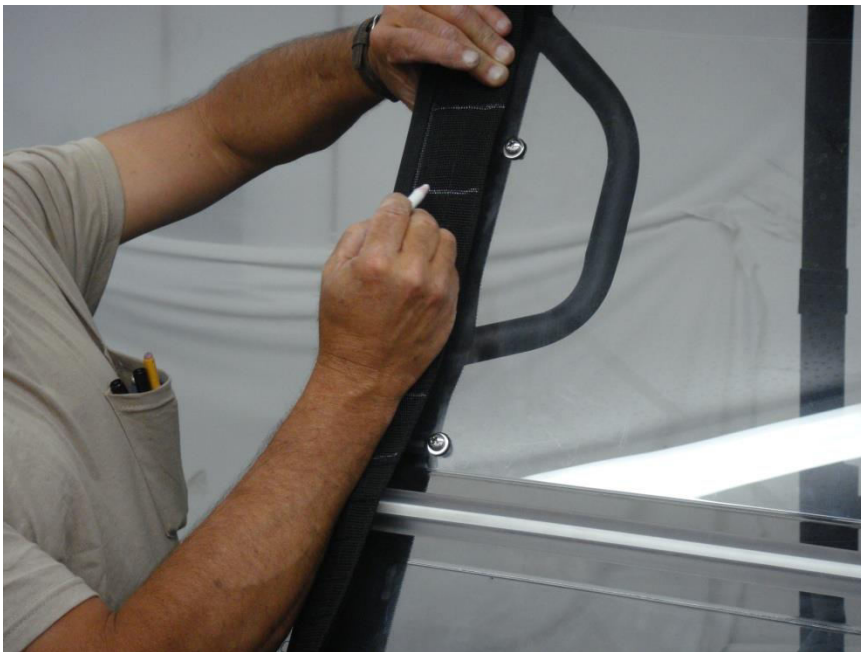
Figure 7.2 - Mark the Windshield Velcro Tabs for hard windshield Clamp locations
