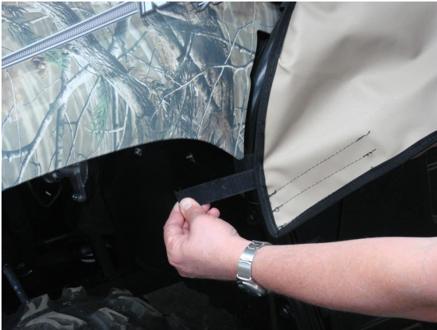
Figure 9.1 - attach Bottom Roll Bar Tabs horizontally around the Velcro Strip and Roll Bar
