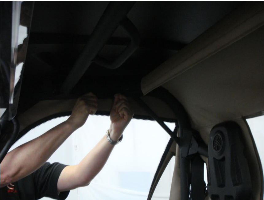
Figure 8.2 – attach 15" Side Roll Bar Cross-member Velcro Tabs
