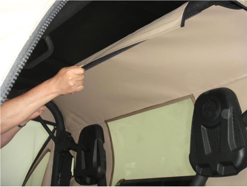
Figure 8.1 – attach 41" Rear Roll Bar Cross-member Velcro Tab
