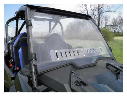
**Step 5:** With the windshield in place, one at a time, wrap the attachment strap around the roll bar and feed the strap through the buckle. Reverse the direction of the strap after going thru the buckle. Pull the strap tight and adhere the hook end of the strap to the loop strap.
