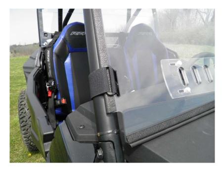
**Step 4:** Hold the windshield to the roll bars. The bubble on the trim along the bottom of the windshield should rest gently on the hood line. Do not mash the bubble flat.
