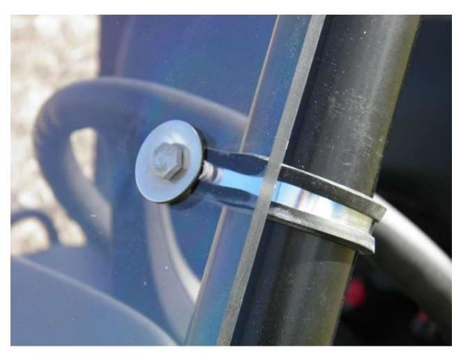
When installed correctly, the flat side of the clamp faces the windshield. The hex head bolt with neoprene washer runs thru the clamp hole opening and secured with a washer and nut on the back side.
