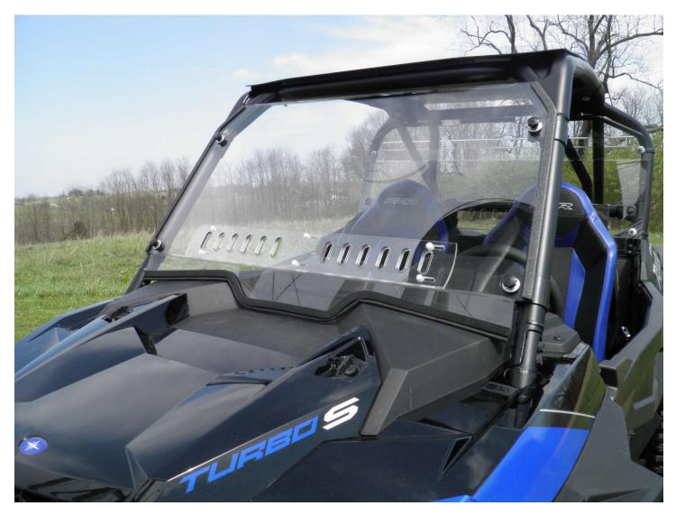
Step 6: When satisfied that the windshield is positioned properly, tighten the two nuts on the back side of each clamp.
