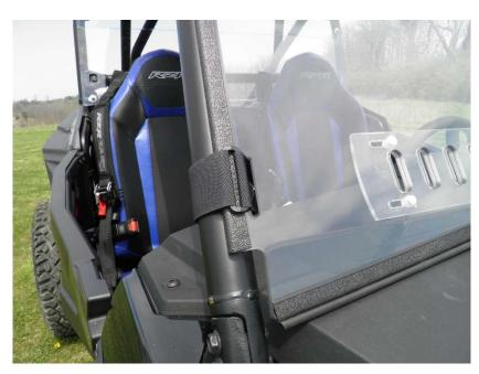
**Step 4:** Hold the windshield to the roll bars. The bubble on the trim along the bottom of the windshield should rest gently on the hood line. Do not mash the bubble flat.
