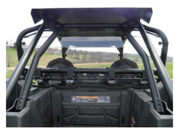
**Step 6:** Assistance may be needed to hold the back panel in place to complete installation. Hold the back panel to the inside of the rear cab frame. Match the bends in the back panel to the contour of the rear roll bars.
