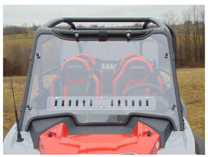
Step 6: When satisfied that the windshield is positioned properly, tighten the two nuts on the back side of each clamp.
