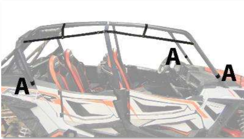
Figure 1: Shows position of Velcro strip A. Velcro will wrap around the roll bar.
