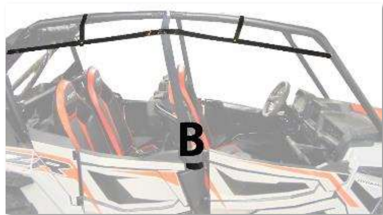
Figure 2: Velcro will be wrapped around the plastic below the front door hinge and notch for the latch on the back door.
