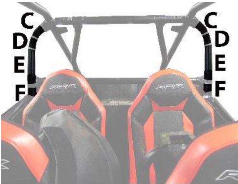
Figure 3: Shows placement of Velcro strips C-F.
