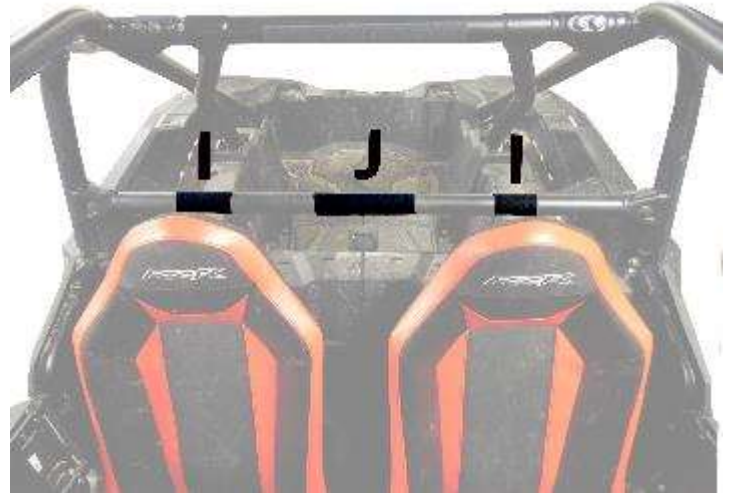
Figure 6: Shows placement of Velcro strip I AND J.
