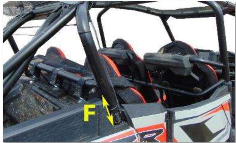
Figure 4: Place Velcro strip between the roll bar and bed of the UTV.
