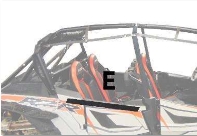
Figure 3: You may cut the Velcro strip where it interferes with the door hinge.
