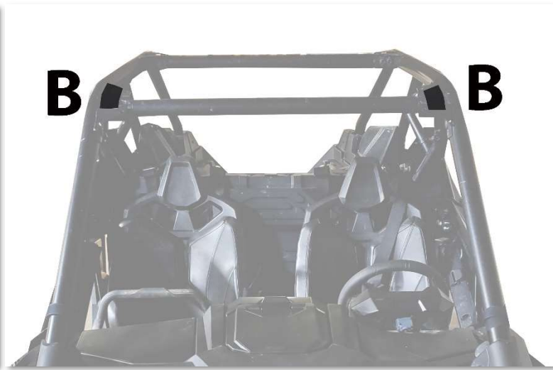
Figure 2: SHOWS PLACEMENT OF VELCRO STRIPS (B).
