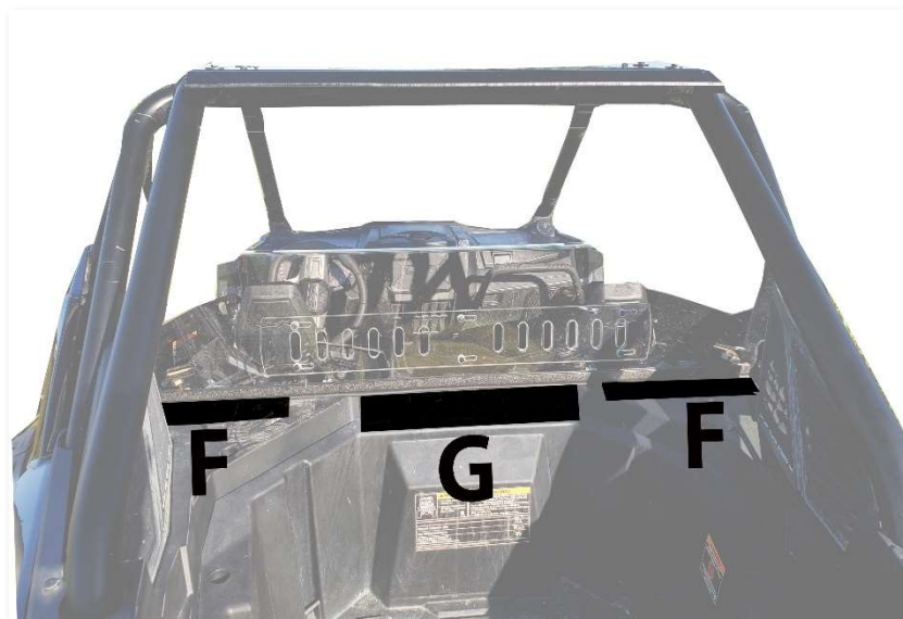
Figure 3: SHOWS POSITION OF VELCRO STRIPS (F,G)
