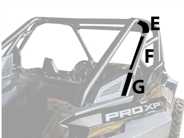
Figure 5: SHOWS PLACEMENT FOR VELCRO STRIPS (E F G). PLACE ON EITHER SIDE.
