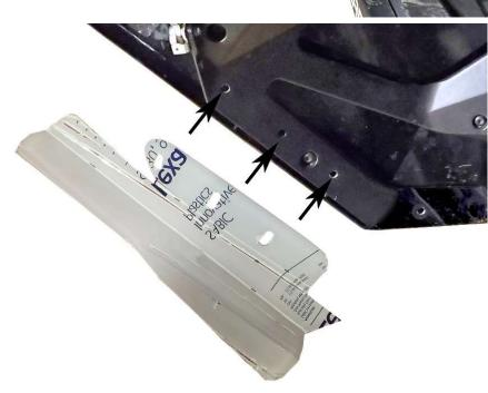
Insert Self Tapping Bolt through the holes in the lexan and then through the factory holes in the door. Use drill to secure. Line up the pointed part of the lower door insert with the corresponding groove in the side insert. Push both parts together and push the trim that is already attached on to the bottom of the insert on to the bottom of the side panel.
