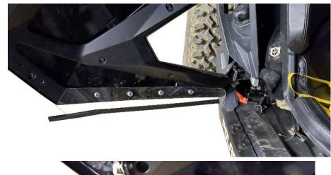
Peel back protective paper enough to expose the holes in the side door insert. Line holes in the panel up with the holes in the factory door.
