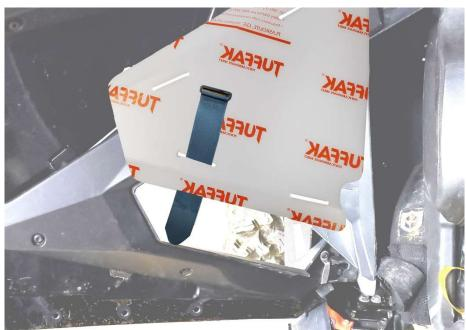
Then insert the 10" strap through the very small opening between the factory door and the plastic cover.
