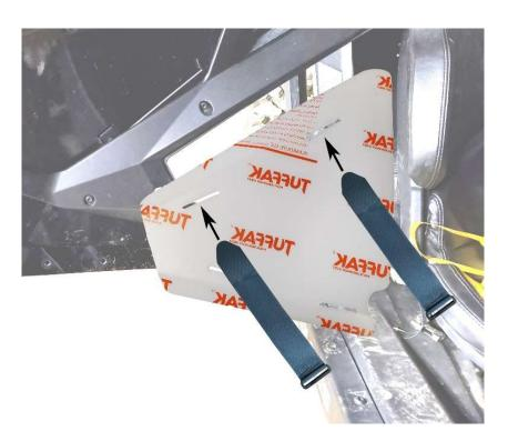
Then insert the 10" strap through the very small opening between the factory door and the plastic cover.
