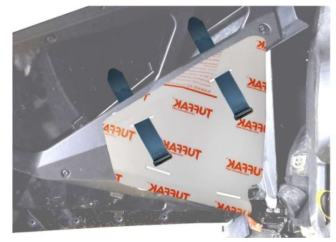
Wrap the end of the 10" strap around the triangle and through the straps buckle. ]
