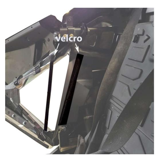
These steps are optional, we have included a soft panel to close up the gap between the triangle and the back of the door. Install Velcro on the inside of the triangle and beside the seat. Attach soft panel and your installation is complete!
