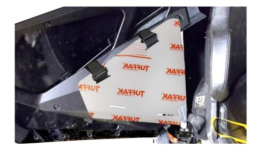
Peel back protective paper enough to expose the slot cut in the triangle. Insert 10" strap, loop facing the triangle, through the slot.
