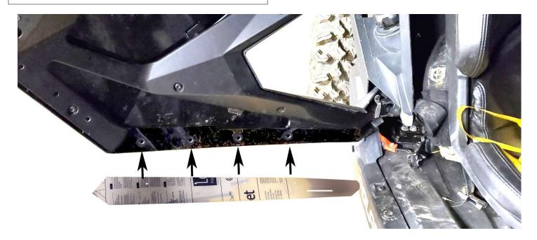
Insert Self Tapping Bolt through the holes in the lexan and then through the factory holes in the door. Use drill to secure.
