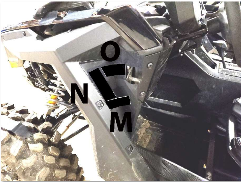
Figure 7: SHOWS PLACEMENT OF VELCRO STRIPS (M N O). PLACE ON EITHER SIDE.
