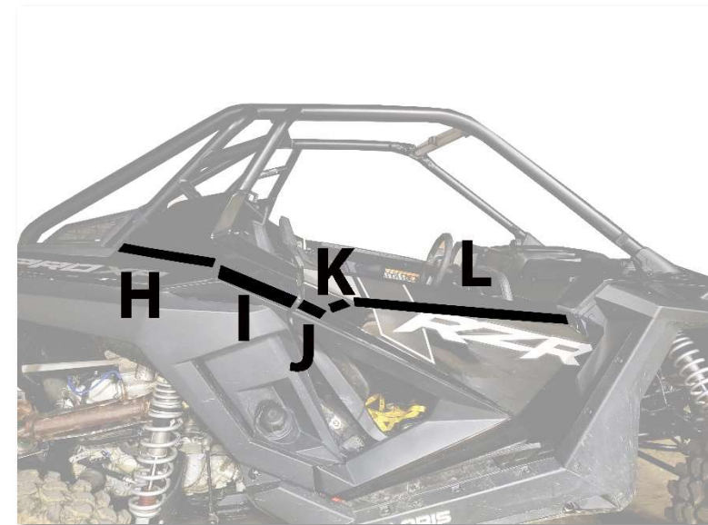
Figure 6: SHOWS PLACEMENT OF VELCRO STRIPS (H I J K L). PLACE ON EITHER SIDE.
