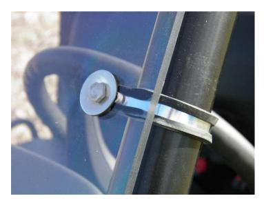
**Step 4:** When satisfied that the windshield is positioned properly, tighten the nuts on each clamp.
