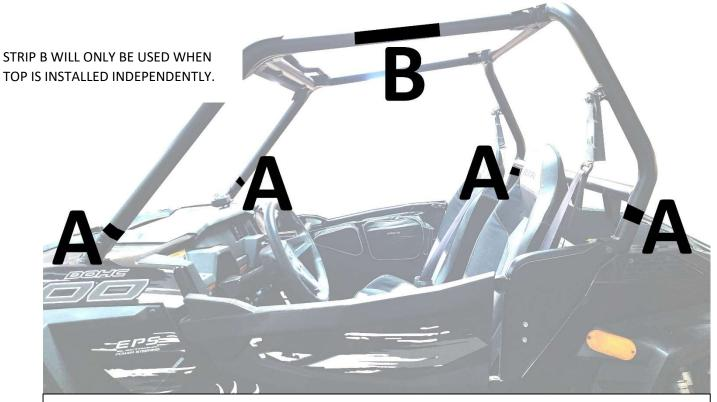
INSTALL THE DOUBLE SIDED STRAPS, SET THE WINDSHIELD BACK ON THE HOODLINE AND INSTALL. THEN PUT THE TOP ON AND ATTACH THE BUCKLES. PULL TENSION STRAP TO TIGHTEN
