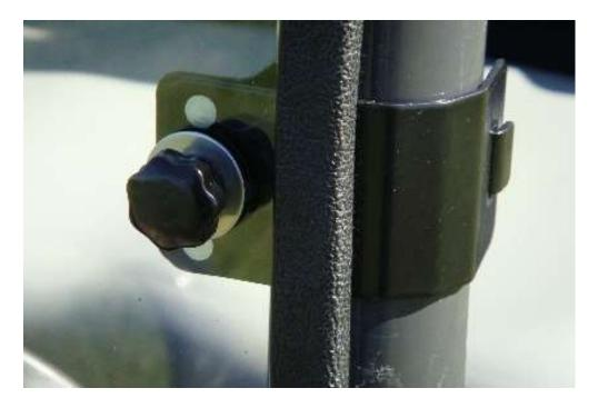
When installed correctly, the flat side of the clamp faces the windshield. The knob bolt with neoprene washer runs thru the clamp hole opening and is screwed into the clamp.
