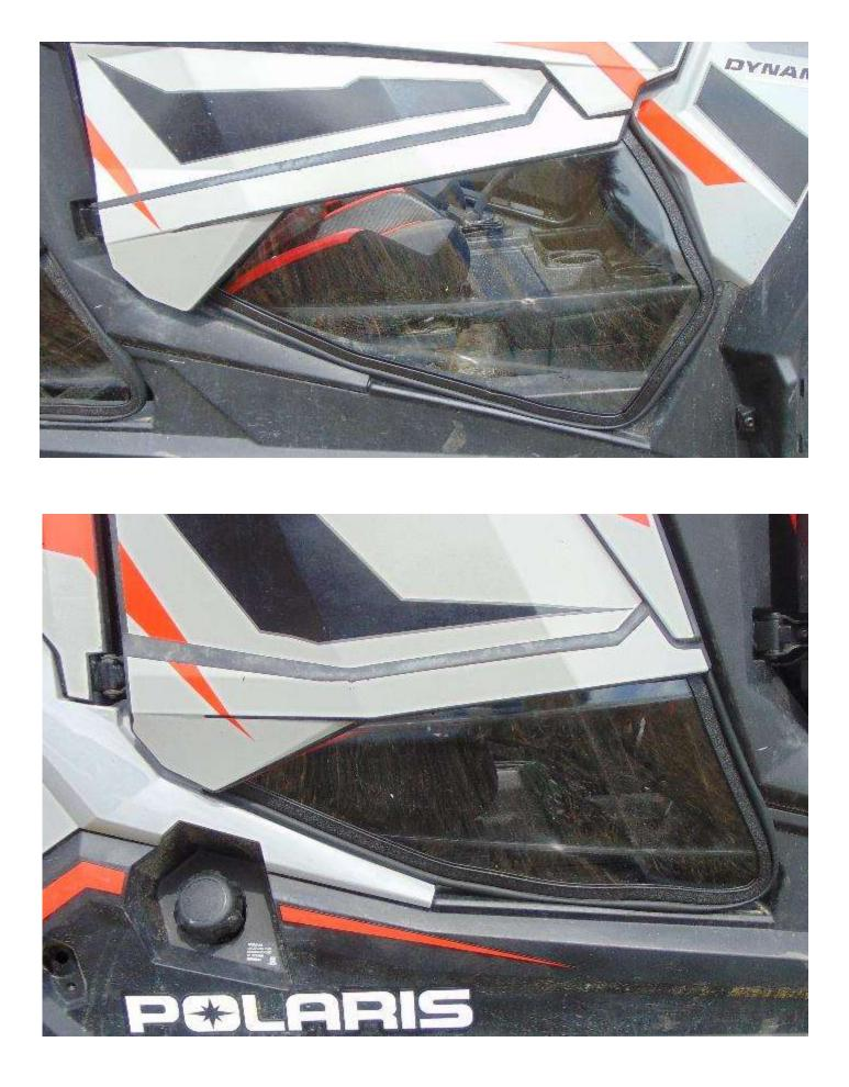
These door panels were not designed to be water tight. Having some small gaps around the trim is normal.
