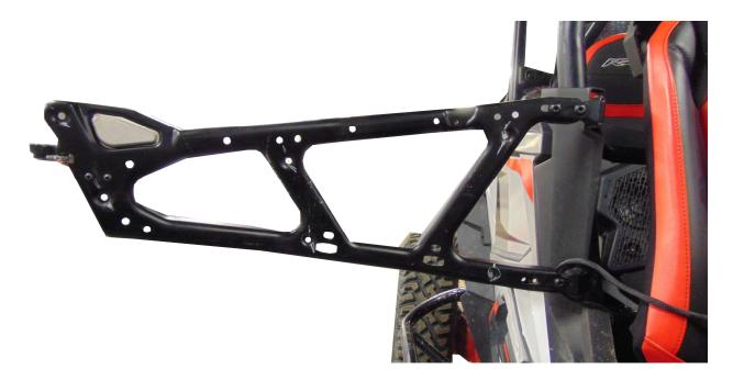
**STEP 2:** Peel back the paper on either side of the bolt holes located in the lexan door panel. These bolt holes are oblong so that you may adjust the panels to the left or right depending on how the panel lines up to the door frame.
