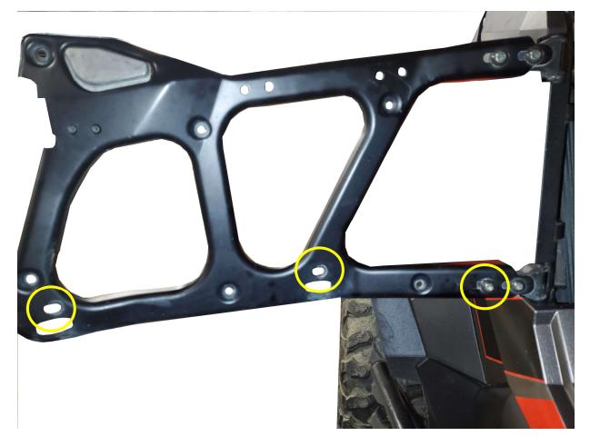
**Step 5:** Install door panel, remove existing bolt (circled) to attach the rear slot to the metal frame, use factory bolt to secure the last slot of your door insert. All other bolts will be installed in the same fashion as the front door panels.
