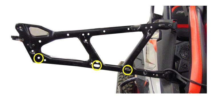
**Step 4:** Remove the plastic panels from either side of the back door leaving only the metal frame. Attach lexan door insert using provided hardware.
