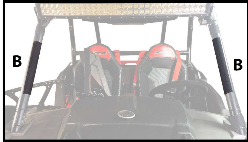
Figure 4: SHOWS POSITION OF 12" VELCRO STRIPS (B)
