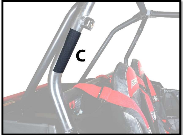
Figure 3: SHOWS POSITION OF 6" VELCRO STRIPS (C)
