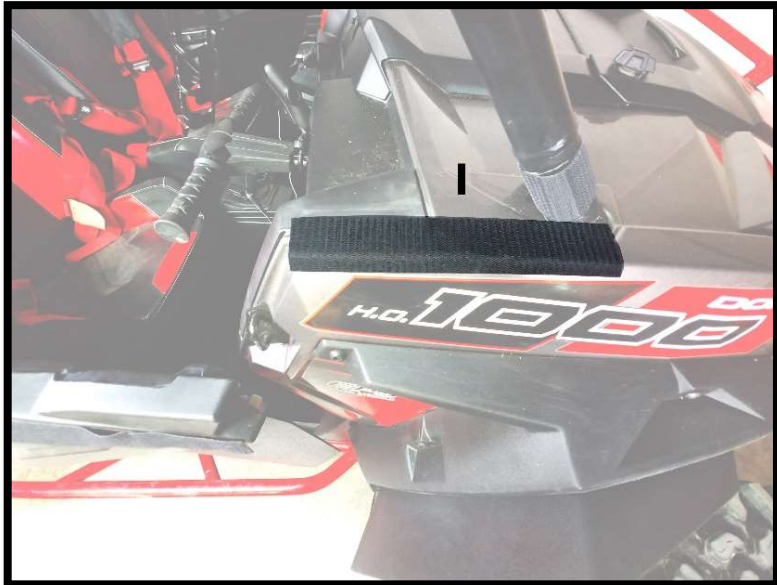
Figure 10: SHOWS PLACEMENT OF 12" VELCRO STRIPS (I). PLACE ON EITHER SIDE.
