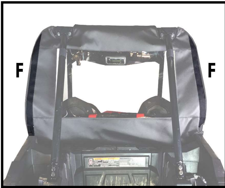
Figure 8: You will attach tabs F to Velcro strips sewn on to the back panel.
