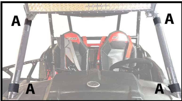
Figure 1: SHOWS POSITON OF 6" VELCRO STRIPS (A)
